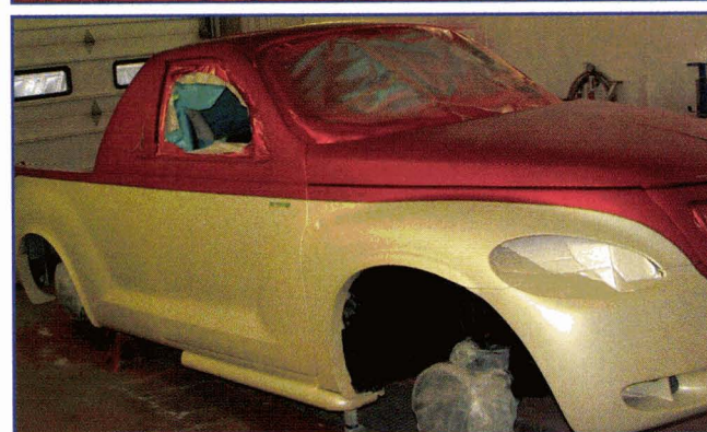
Photos 10 and 11: The front of the hood and the side of the truck before it's clearcoated. You can barely notice the striping, and believe me, there's plenty on the vehicle! This job took about two hours to complete. I had a great time at Brut Manufacturing, and I'm anxious to see how Lynn Neiss and the Cruiser do at SEMA!
