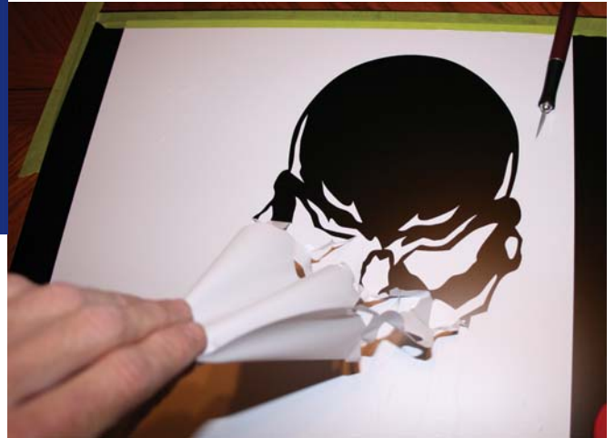
After removing the application tape, peel the excess material away from the design (also known as 'weeding'). Below: The final stencil is ready for paint.
