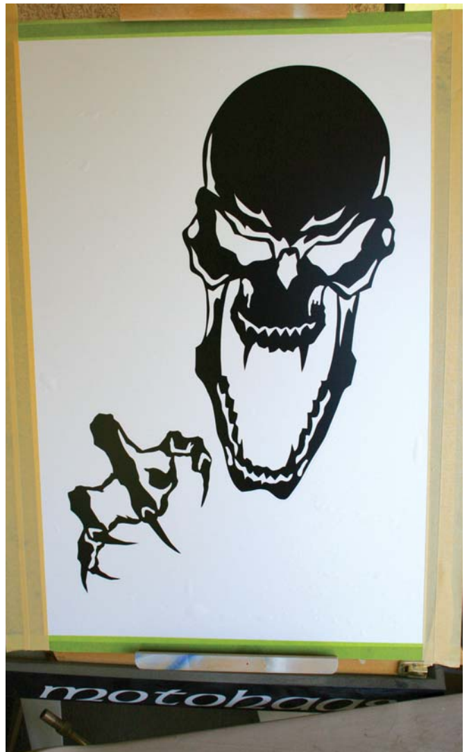
After removing the application tape, peel the excess material away from the design (also known as 'weeding'). Below: The final stencil is ready for paint.
