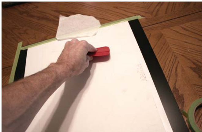
After transferring the stencil using application tape, use a squeegee to smooth down the stencil.
