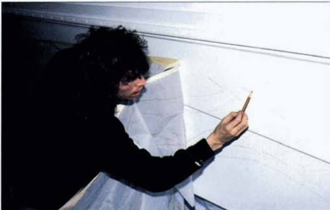
4. We then traced one side of the hull onto tracing paper. Flipping it to the other side, we copied the trace onto the hull.
