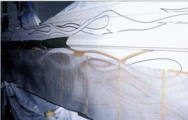
5. After we taped up the big areas with paper, we then cleaned the boat again with the degreaser.
