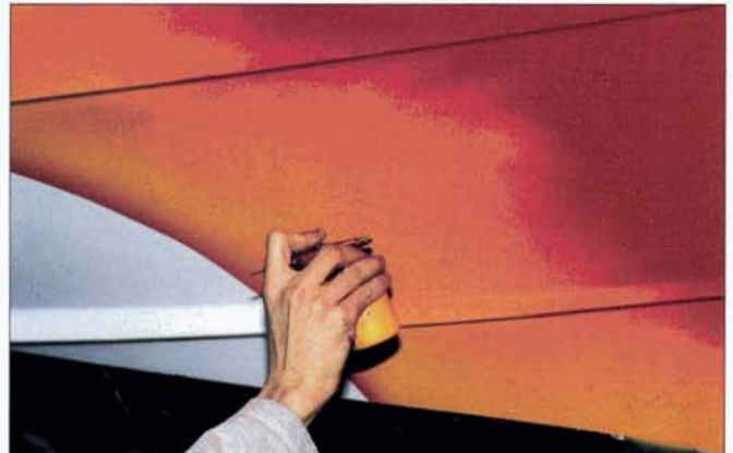
8. We unmasked and added some final highlights. The lines that we left with the 1/4-inch 3M tape disappeared when we pinstriped the flames. Flames generally need to be pinstriped in order to give a finished look.
