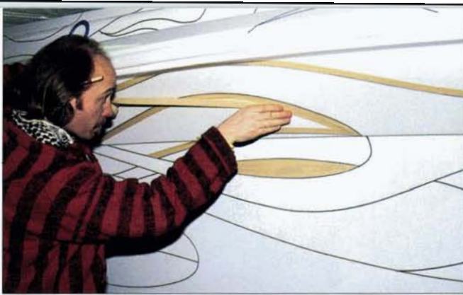
3. We then used painter's masking tape to tape up the areas we didn't want sprayed.
